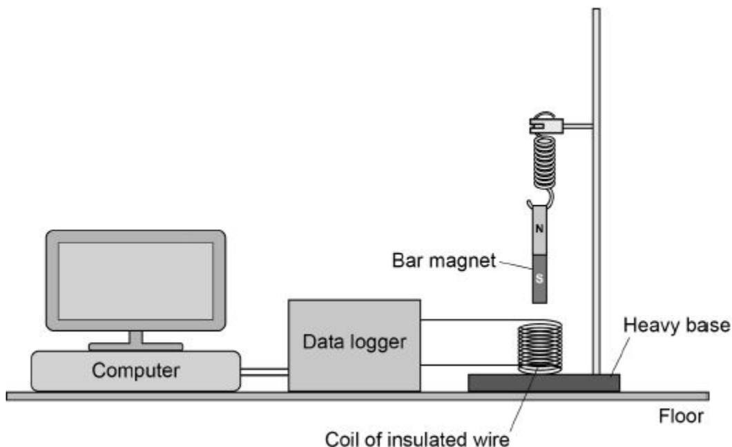
To test that the seismometer works, the student pushes the bar magnet into the coil and then releases the bar magnet.
