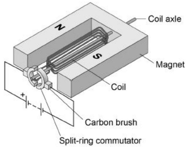
When there is a current in the coil, the coil rotates continuously.
